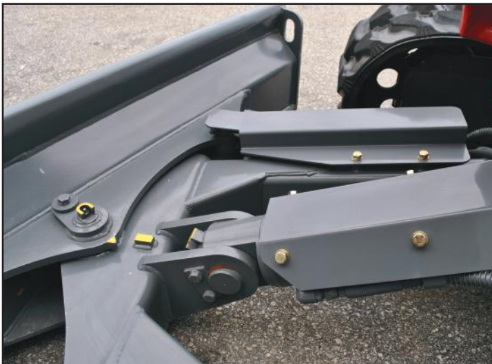
Angle Blade with Reversible Bolt On Cutting Edge
